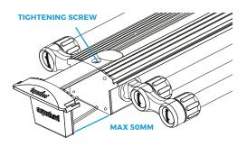
If required the AquaLumi Universal can be extended to fit your aquarium. Simply unscrew the plastic screw located on the top of each of the end caps, slide out the extension brackets to the required length and tighten the screw back up.
