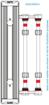
STEP 1 Place two screw caps onto each tube as shown in the below illustration.
