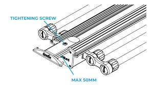
If required the AquaLumi Universal can be extended to fit your aquarium. Simply unscrew the plastic screw located on the top of each of the end caps, slide out the extension brackets to the required length and tighten the screw back up.
