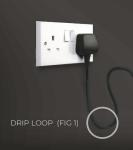
As with all aquarium electronic equipment, make sure you have a drip loop to prevent the socket or plug from getting wet. As shown in (fig 1), opposite, the part of the power cable lying below the level of the socket is used to prevent the water entering the socket
