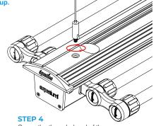
Screw the threaded end of the suspension fitting onto the receiving hole on each end of the lightng system.
